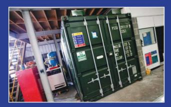
'AirTech' container shot blast rooms are a robust, energy-efficient and low cost solution for all forms of enclosed, freestanding shot blasting operations.
