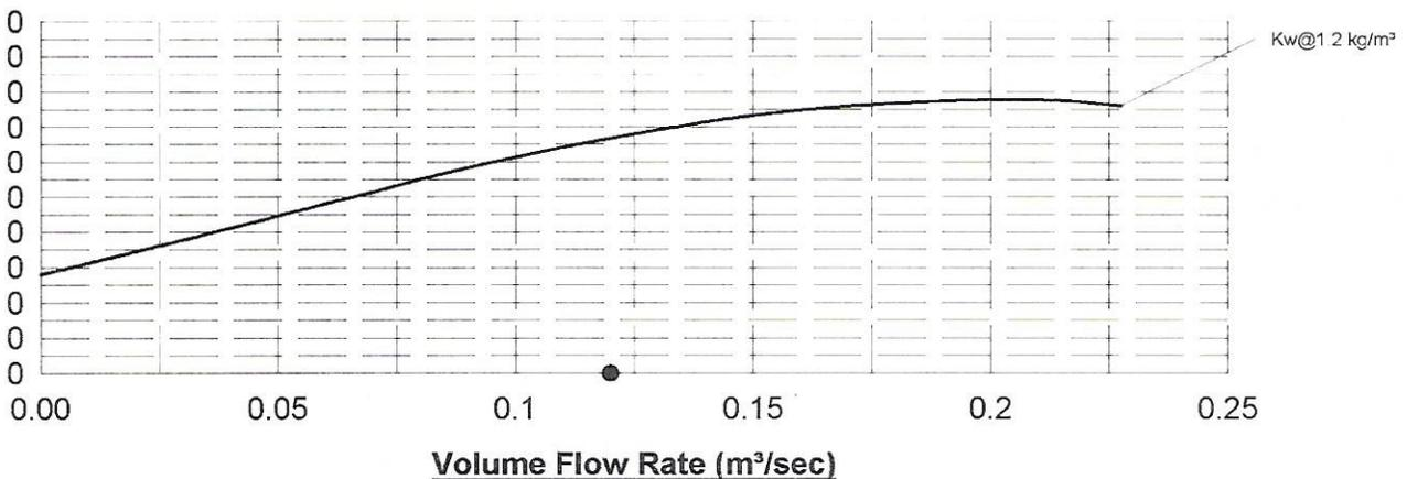
Power values at 1.2 Kg/m<sup>3</sup> At operating point :-0.0 Kw / Peak:-0.04 Kw / Closed:-0.01 Kw
