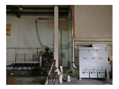
The automatic filter cleaning systems shakes down the filters on shutdown with easy removal of dust from the collection bins which also have wheels for easy movement.
