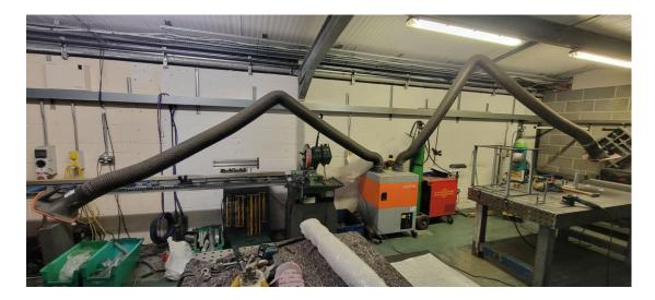
Two stage filtration ensures that fumes and dust from welding are contained and clean air is returned to the working area.
