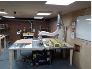
Our four bin extractor makes disposing of wood dust easy due to its quick clip system.
