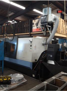
Mist and smoke are extracted through the hose and are taken through multiple filter stages. The conical main filter coalesces large particles on impact; then uses the wind shear principle to separate finer mist with further separation in the internal mesh layers.
