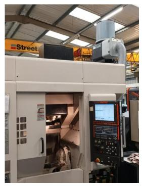
Mist and smoke are extracted through the hose and are taken through multiple filter stages. The conical main filter coalesces large particles on impact; then uses the wind shear principle to separate finer mist with further separation in the internal mesh layers.
