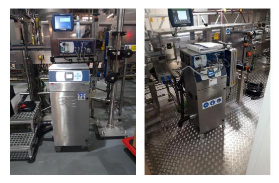
The "plug and play" extractor contains two stage filtration which protects the user and removes harmful smoke and fumes which are held for safe disposal by the units.
