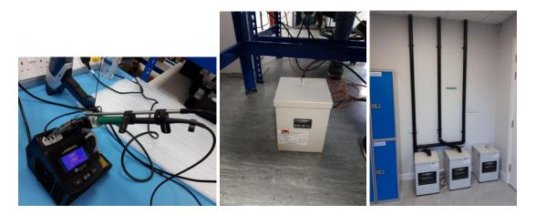
Two stage filtration protects the user and removes harmful smoke and fumes which are held for safe disposal by the units.
