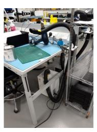
The two stage filtration removes smoke and fumes from the process and holds this in the filters for disposal.
