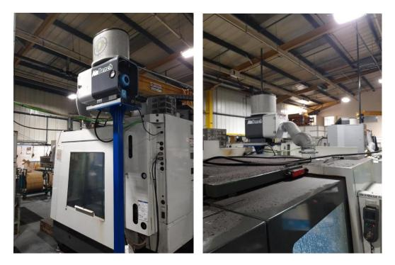
Mist and smoke are extracted through the hose and are taken through multiple filter stages. The conical main filter coalesces large particles on impact; then uses the wind shear principle to separate finer mist with further separation in the internal mesh layers.
