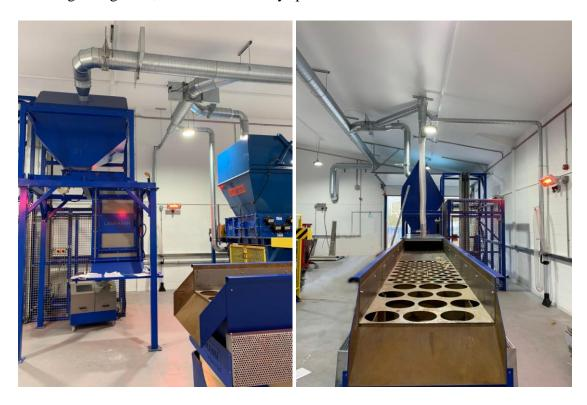
Two vacuum points were added to the system to allow for housekeeping duties.
