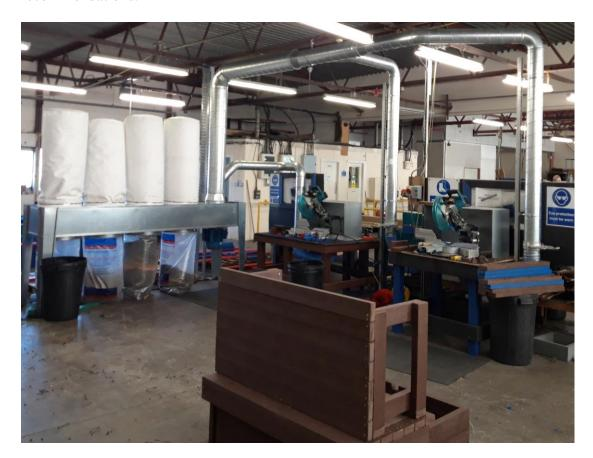
The four bag dust extractor was selected as the customer wanted 100% usage of all chop saws. Even flow through the extraction system was ensured via balancing dampers and transport velocities of dust through the ducting were in excess of HSE recommendations.
