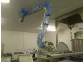
Each Dust Extraction Arm is moveable through 360° to ensure that an operative could move between multiple working stations with an adjustable hood.
