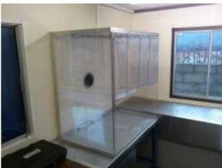
The Dust Extraction System is fitted with an automatic shaker mechanism to ensure no particles are lodged on shutdown which reduces operator dependency. Four collection bins ensure easy, clean and safe access to the waste for disposal.
