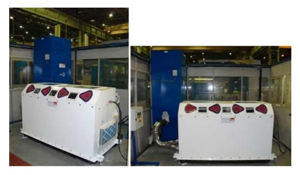
The dust extraction system is fitted with multiple polyester needle felt, anti static, micro deniar filter elements. A secondary filtration system incorporates a Hepa filter and a 100 litre metal waste bin to ensure quick and easy removal of the waste.
