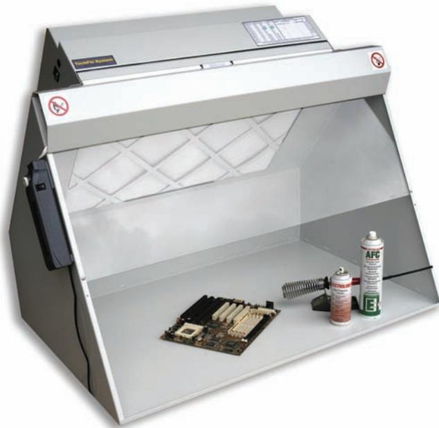
NOTE: These units are recirculatory; i.e. filtered air is exhausted back into the workplace
