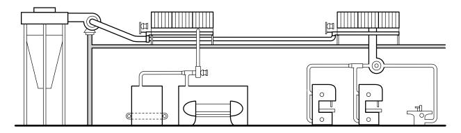
Figure 2 Typical dust extraction system
