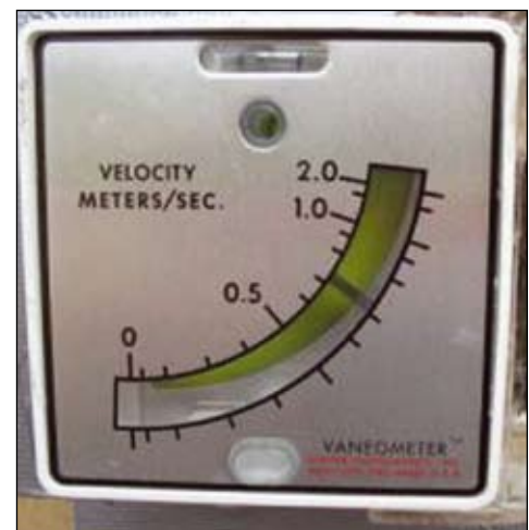
Figure 15 Example of a 'swinging vane' fitted to a spray room
